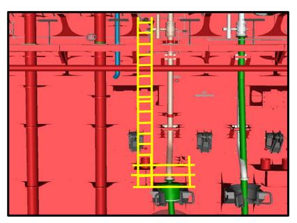
2m x 2m Platform Scaffold for flange inspection, alignment, flange management, leak testing and coating application.
