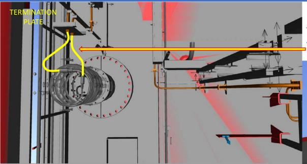
Tie-in of Flexibles and cable connections from TUTU to Umbilical Terminations.
